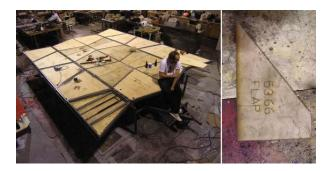
Figure 2 - Fabrication of the Mobile Stage (L) and CNC cut Jig for laying our and welding the trapezoidal frames (R)
